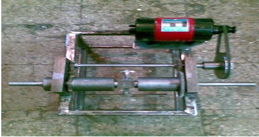
Fig. (2). The prototype of Capstan mechanical power amplifier
